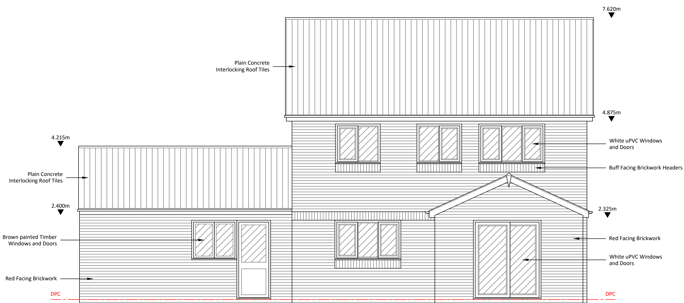
2.3 Existing Rear (North) Elevation Scale 1:50
